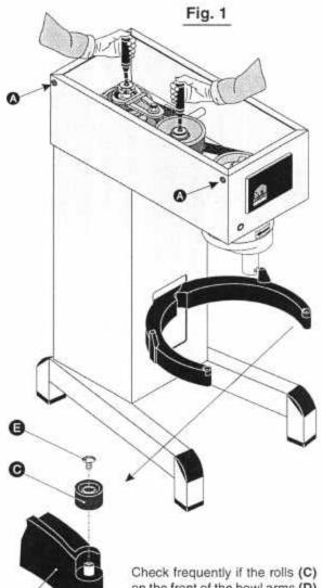
on the front of the bowl arms (D) can rotate. They can be cleaned by removing the screw (E) whereafter the roll can be pulled up. Wash the shaft and the roll in lukewarm water.
